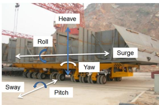
Figure 1 – Identification of the six degrees of freedom of a platform vehicle. Source: adapted from Unta, 2015.
