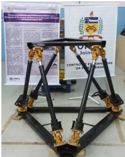
Figure 7 – Stewart Platform prototype under development at LGI/UFSC.
