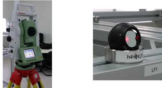
Figure 3 – Robotic total station (left) / Spherical mounted reflector - SMR (right).
