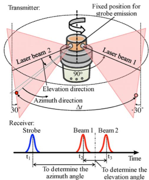
Figure 2 – Azimuth and elevation angle determination of a transmitter-receiver vector. Source: adapted from Depenthal et al., 2009
